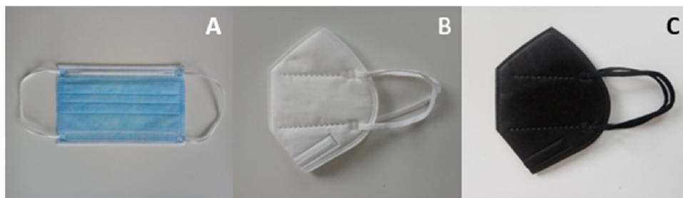
Figure 1. Images of masks used for this investigation. (A) Omnitex (showed as an example of all three Type IIR DPFMs), (B) Baltic (same features as Soyes), and (C) Geji (both FFP2 type).
