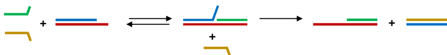
Figure 14.2 Allosteric toehold mechanism. A first input invades the target duplex, revealing a new domain used by the second input in a subsequent strand displacement reaction.
