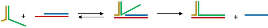
Figure 14.4 Associative toehold mechanism. The helper strand (orange) facilitates the strand displacement reaction by bringing the invading strand (green) into proximity to its target domain (red).
