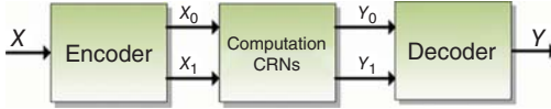
Figure 3.5 The system performing encoding, computing, and decoding signals in CRNs. Source: From Salehi et al. [17]. Reproduced with the permission of American Chemical Society.
