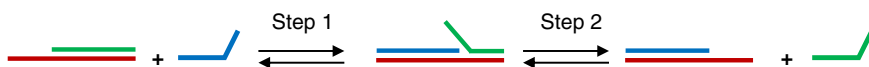
Figure 14.6 The toehold exchange reaction. The process is fully reversible via reverse toehold binding and strand displacement.
