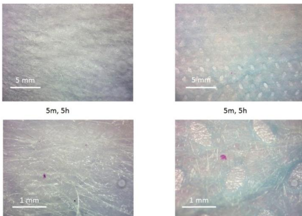
Figure 9. Setting 3: Microscopic image of the masks after exposure for 5 h at a distance of 5 m from the face (a person without a mask reading a book aloud) in a room (40 m 2 ) ventilated every hour: Left pictures = inner side of the mask, Right pictures = outer side of the mask, single clusters of microorganisms (coloured intensely pink) are visible.
