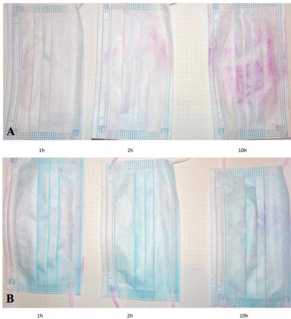
Figure 5. The photographs show the inner and outer surface of stained masks from Setting 2 after different exposure times: A=inner part, white, B=outer part, blue.
