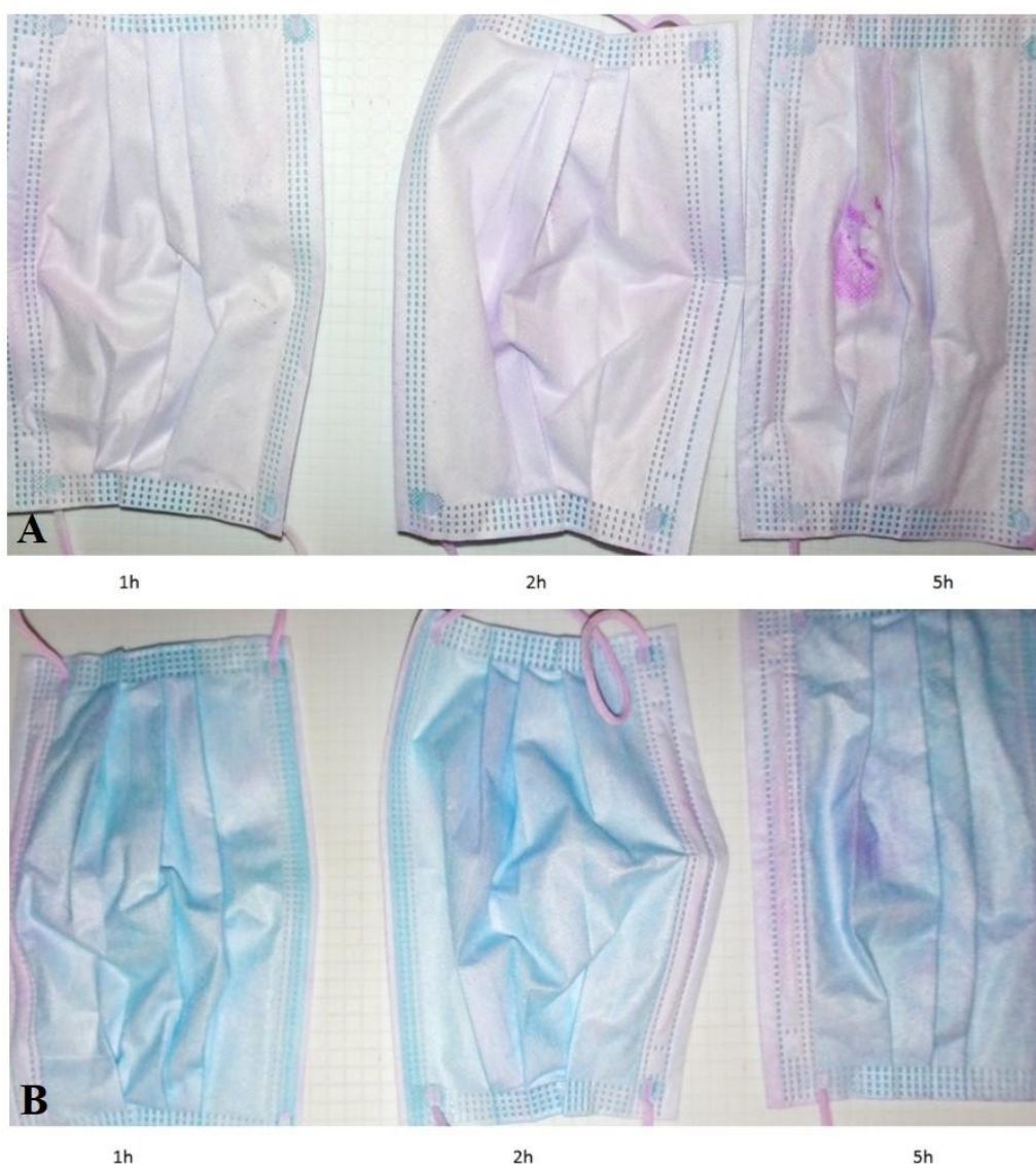
Figure 3. Macroscopic images of stained masks from Setting 1 (masks worn). A=inside, B= outside view of the mask.
