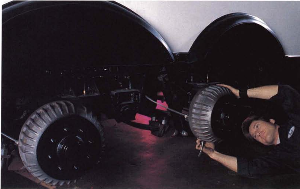
Above, the principal product of Thousand's Wolverine Western Corporation: an advanced brake drum featuring a ribbed hub, a spinoff from rocket engine nozzle design technology. The ribs reinforce and cool the drum, helping to prevent a shape distortion known as "bellmouthing" that adversely affects braking efficiency. At left, a mechanic adjusts the brake shoes.
