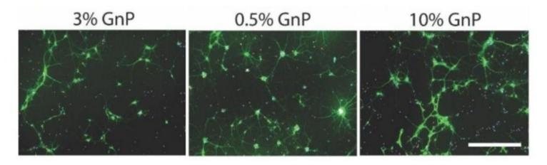
"Here we have developed a polymer matrix **P(3HB)** (hiroxybutyl) **with GnP** (graphene) that results in increased electrical conductivity of the matrix. The P(3HB)/GnP compound promoted neuronal growth and maturation."
