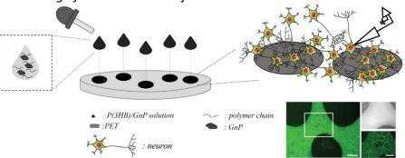
incorporating graphene nanoplatelets (GnP). The growth, network formation and functionality of primary neurons in polymeric supports of **poly(3-hydroxybutyrate)** [P(3HB)] functionalized (glued) with GnP (graphene)"
